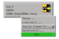
The source correlation tool set correlates the logic analyzer's address label with a line of high-level source code whose address, symbol name, file name, and line numbers are described in a symbol file downloaded to the logic analyzer (see "To load object file symbols" on page 93).
