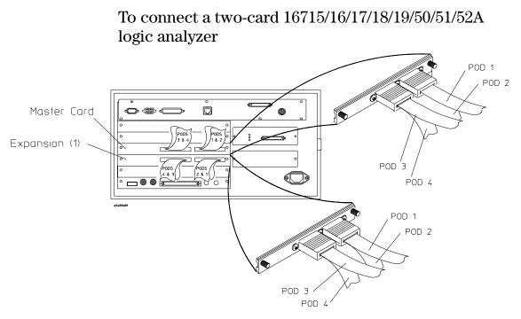
Use this table to connect cables from the Agilent Technologies 16715/16/17/18/19/50/51/52A logic analyzers to the connectors in the target system.
