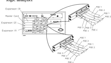
To connect a four-card 16715/16/17/18/19/50/51/52A logic analyzer
