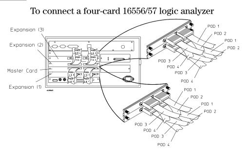
Use this table to connect cables from the four-card Agilent Technologies 16556/57 logic analyzer to the connectors in the target system.
