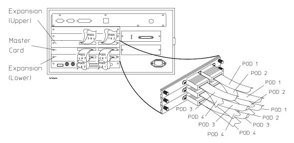
To connect a three-card 16554/55/56/57 logic analyzer
