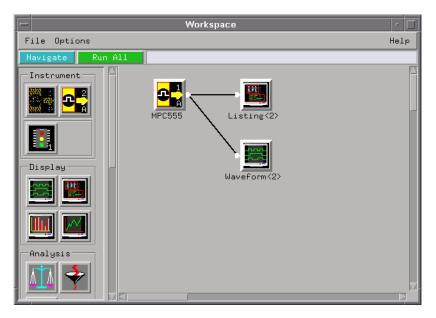
This setup is appropriate for debugging hardware. When you're debugging software, you'll probably want to use the trace reconstruction tool (see "Displaying Data from the Trace Reconstruction Tool" on page 112).
