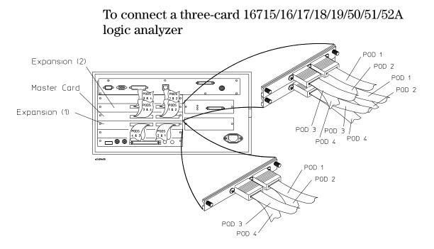
Use this table to connect cables from the Agilent Technologies 16715/16/17/ 18/19/50/51/52A logic analyzers to the connectors in the target system.
