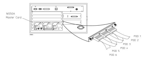
To connect a one-card 16550A logic analyzer
